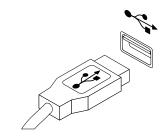
Figure 48. Connecting the USB keyboard or mouse
